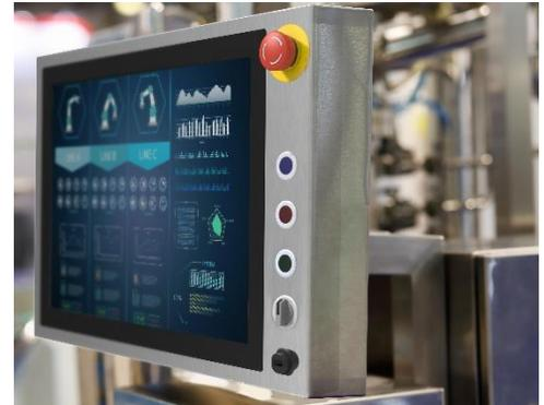
*User-defined function push-buttons and rotary switch on front panel*
