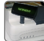
Rotatable VFD client display
